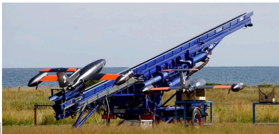
A catapult used for testing drones
